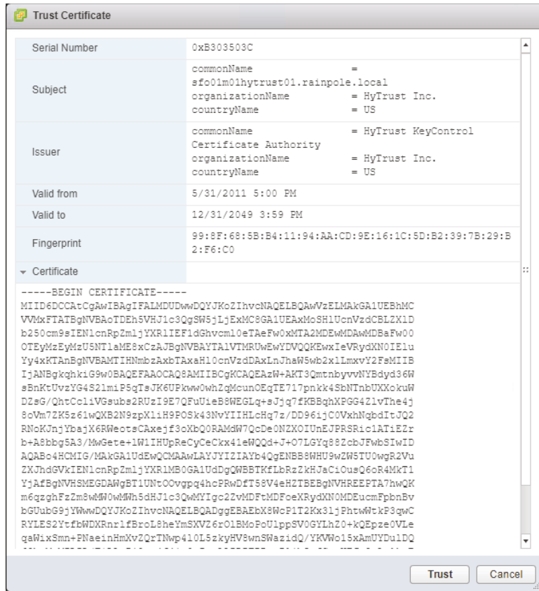
FIGURE 8.18 When prompted to trust the KMS, review the serial number, the common name, and the fingerprint on the presented certificate to ensure everything matches the certificate on actual KMS.
