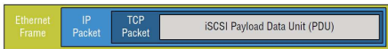
Figure 6.12 Using iSCSI, SCSI control and data are encapsulated in both TCP/IP and Ethernet frames.
